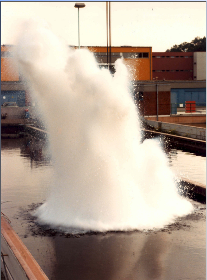
150 l of LN 2 spilled on water
